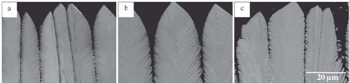
Fig. 1 Scanning electron micrographs of EB-PVD TBCs cross sections manufactured at different temperatures and rotation speeds conditions. (a) "Intermediate," 950 °C/12 rpm. (b) "Coarse," 1000 °C/3 rpm. (c) "Feathery," 850 °C/30 rpm
